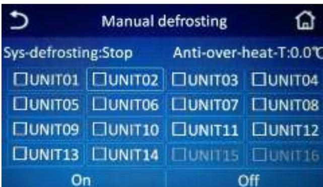
Enable the defrosting function of the selected unit. When “”turns to “”, it indicates manual defrosting function for this unit has started as shown in the figure below.
