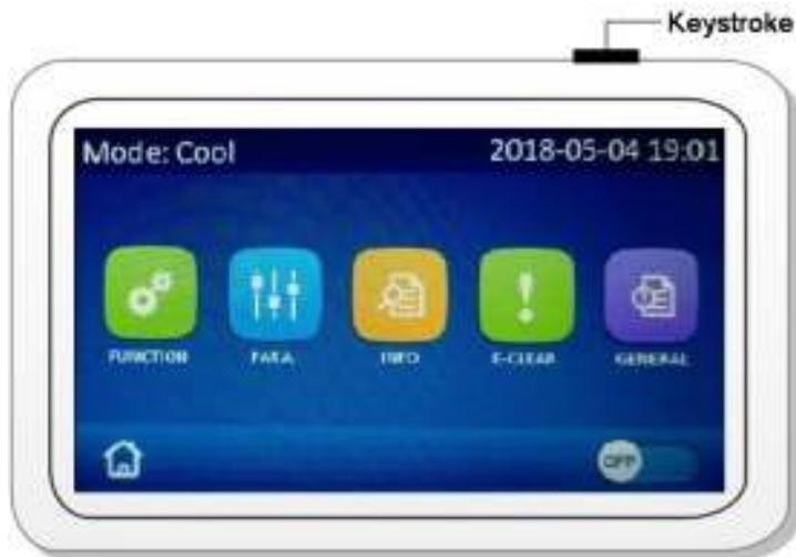
It uses the capacitor type touch screen for information input. The effective area for touching indicates the rectangular black area when the backlight of the control panel lights off.
