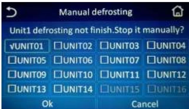
By pressing “**OK**”, manual defrosting will be deactivated, with “”changed to “”.
