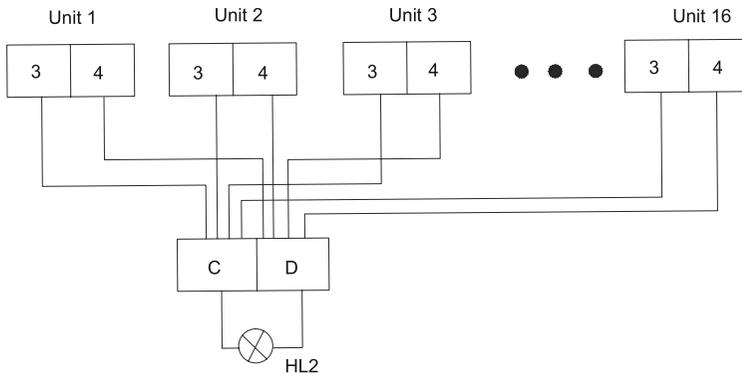
When it is required to display errors of several units, the wiring terminals (3, 4) of each unit should be wired to the wiring terminals HL2 (C, D) of the error indicator. (If it is required to display the error of each unit independently, then the error indicator of each unit should be wired independently to the corresponding error output wiring terminals (3,4) of each unit.)
