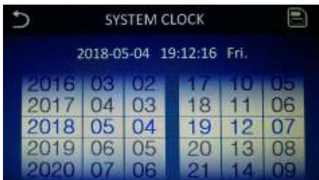
The setting value for the system clock can be changed by the sliding the blue digits. Then, by touching the saving icon, this setting will be saved and rightly take effective. While, by touching the back icon, this setting will not be saved and the controller will back to the general setting page.
