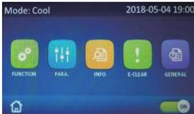
(3) At the homepage and menu page when the unit is "ON", by touching "ON/OFF", the control panel will access to the following page.
