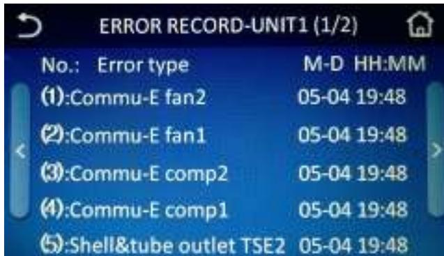
At most 10 pieces of error records can be saved for each unit. When it exceeds 10, the earlier ones will be deleted, which will not affect the error records of any other units.
