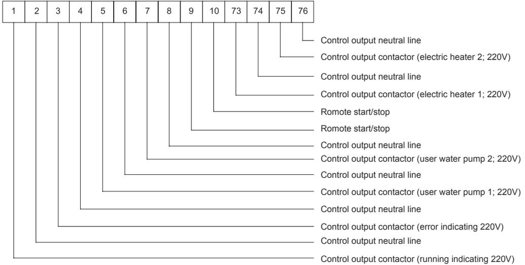
Note: the output control lines of the AC contactors for the running indicator, water pump 1, water pump 2, auxiliary electric heater 1, auxiliary electric heater 2 can be wired to the corresponding wiring board of any one unit, while those for the error indicator and external passive contact switch should be wired to the corresponding wiring board of all units as shown in the figure below.
