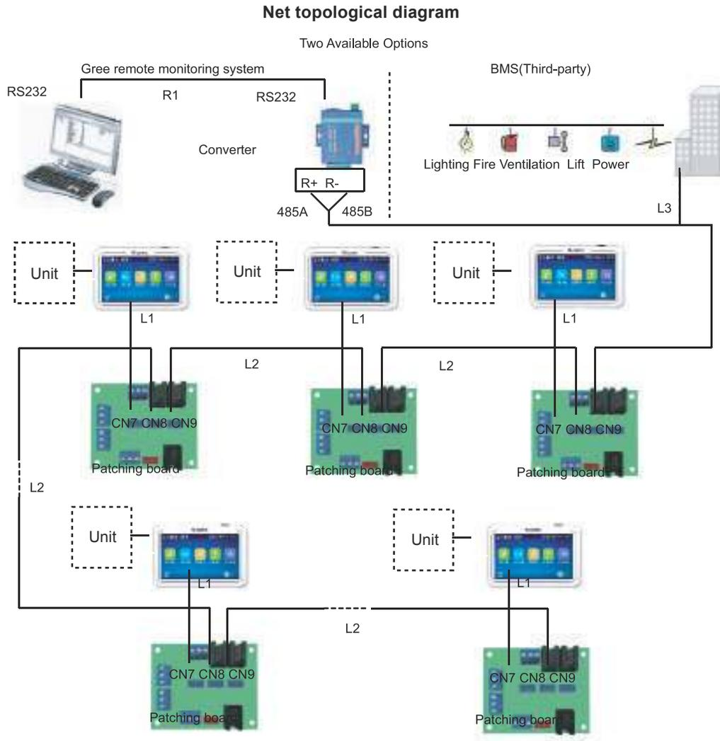
Note: the system as shown in the figure above consists of 1~16 single units depending on the actual demand of the project.
