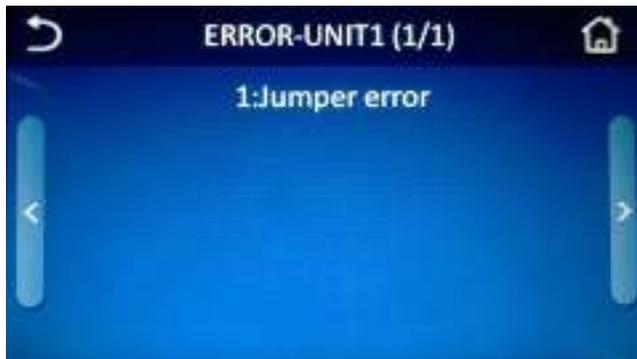
When the quantity of error exceeds 5, by touching the last or next page icon, the desired error can be checked.
