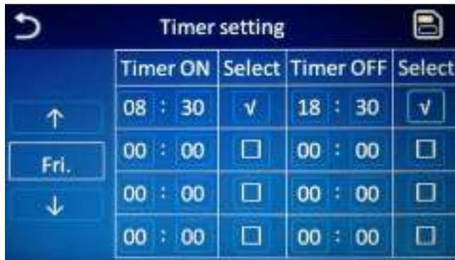
After that, press the saving icon at the upper right corner to save this setting, or press the back icon at the upper left corner to give up this setting.
