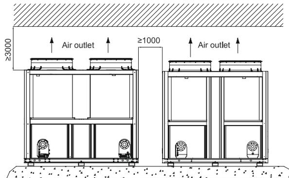
Note: Shock pads (prepared by clients) should be fit to unit bases and fixed with screws to the ground or roofs.
